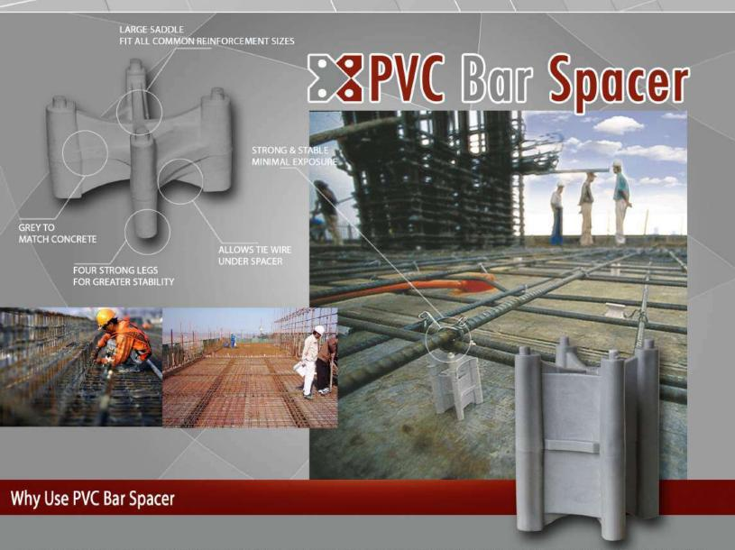
The Atlanta PVC Bar Spacer has been designed to support both mesh and large bars in suspended decks, precast beams and panels, and tilt-up applications. As an alternative to wire chairs and concrete blocks in several applications, the Atlanta PVC Bar Spacer are lighter, offer dual heights and ahve no rust problems.
